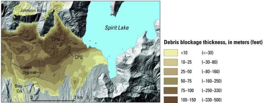
**FIGURE 2.5** Debris blockage thickness shown on topographic model derived from 2009 LIDAR survey. The debris thickness contours run along the old North Fork Toutle River in the northeast-southwest direction. SOURCES: Map derived by Adam Mosbrucker, USGS. Original data from Glicken et al., 1989.
