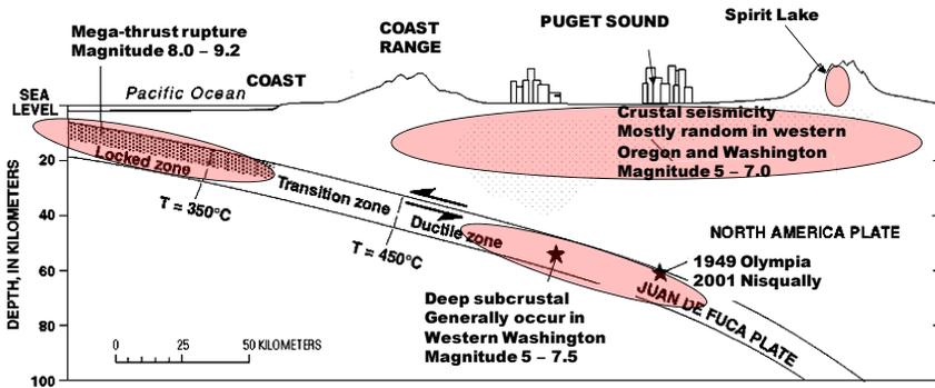
**FIGURE 4.3** Schematic map of seismic sources in the vicinity of Mount St. Helens. SOURCE: USACE, 2016b.
