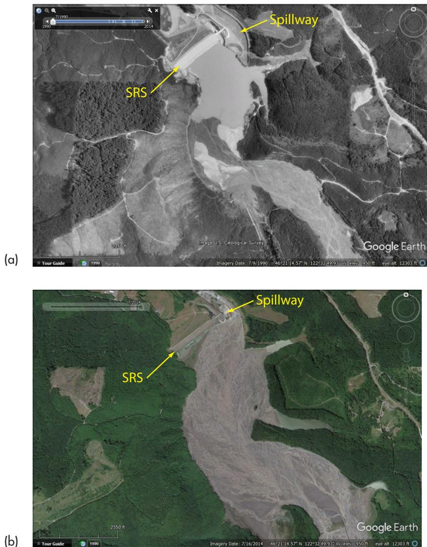
**FIGURE 2.13** Aerial view of the SRS and sediment plain taken both in (a) July 1990 and (b) July 2014. Note the increase in the size of the sediment plain. The SRS, which is approximately 2,000 feet in length, is the northeast-southwest trending linear structure in the upper center of the figure. SOURCE: Google Earth.
