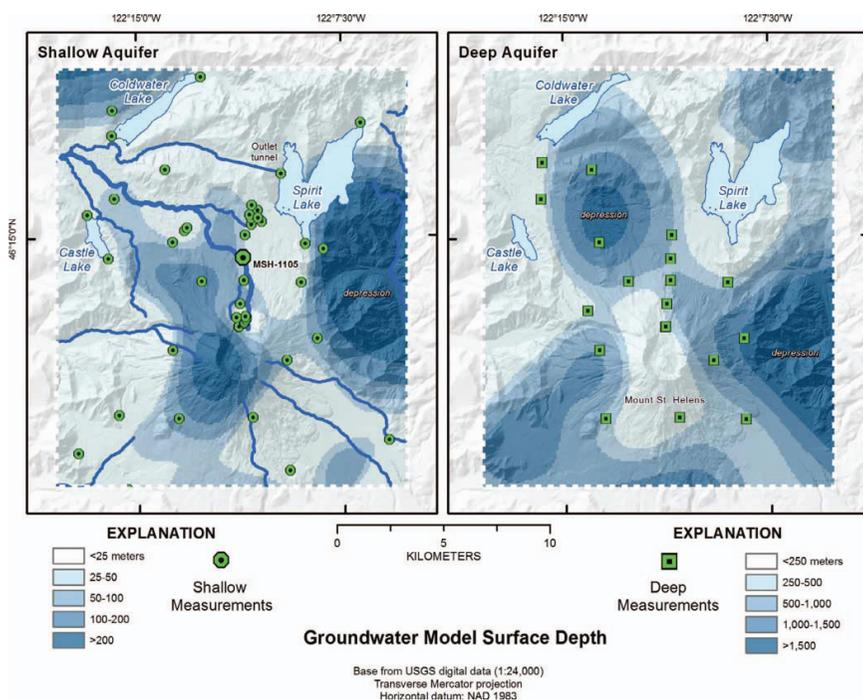
**FIGURE 2.9** Groundwater surface depth from modeling and geophysical data. SOURCE: Wynn et al., 2016. The following material from the *Journal of Environmental and Engineering Geophysics*, 2016, is published with the permission of the Environmental and Engineering Geophysical Society. All copyright privileges remain with the EEGS. This material cannot be copied or used without the express written permission of the EEGS.
