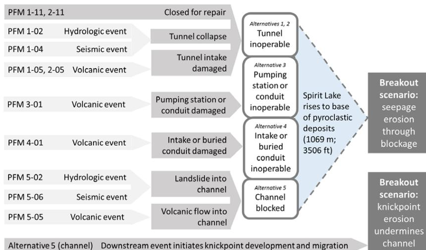
**FIGURE 5.1** Schematic depiction of potential failure modes, outcome of failure mode on infrastructure, and ultimate potential consequence of outlet system failure. SOURCE: Grant et al., 2016a.
