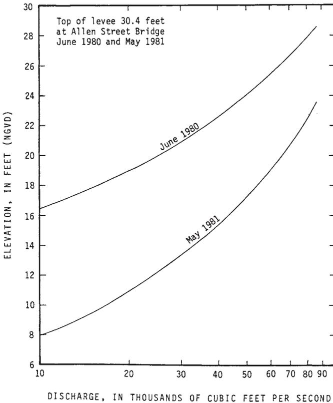
**FIGURE 4.2** Elevation-discharge curve for the Cowlitz River and Kelso-Longview, Washington. The June 1980 curve represents the post-eruption but pre-dredging condition of the river. By May 1981, dredging had lowered the bed of the river and correspondingly the elevation of the river surface. SOURCE: Lombard, 1986.
