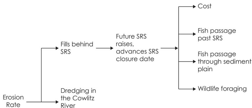
**FIGURE 8.1** A simple influence diagram showing how the erosion rate of sediment might be linked to specific phenomena. Detail in this example is provided for only one phenomenon; others would also have to be diagrammed. NOTE: This diagram does not represent a recommendation; the resulting diagram following an actual discussion may be different.
