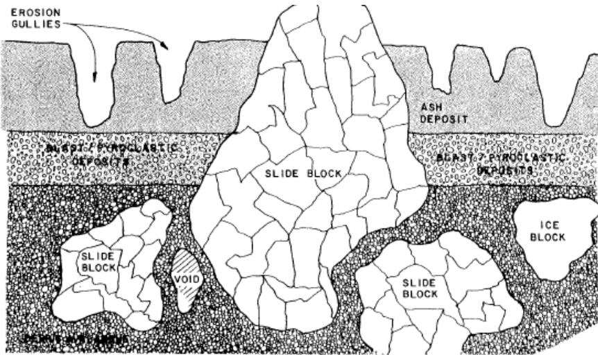
**FIGURE 2.6** Idealized cross-section of the Spirit Lake blockage. The debris blockage also includes pits resulting from the melting of blocks of ice from glaciers located on Mount St. Helens and entrained in the debris slide. SOURCE: USACE, 2016a.
