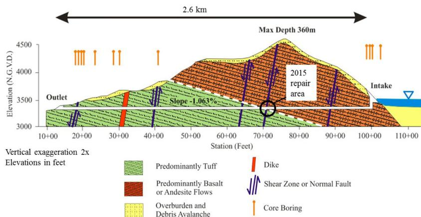
**FIGURE 2.10** Geologic profile along tunnel. Left is west; right is east. There are five mapped shear zones shown. The location of the 2015 repair area is shown. This tunnel was deformed at the contact between predominantly tuffaceous and hard rock materials along the Julie and Kathy L. shear zone. SOURCE: Britton et al., 2016a.
