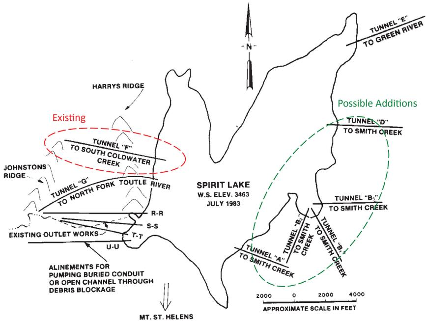
**FIGURE 5.2** Original suggested tunnel alignments. Existing tunnel alignment (circled in red) drains Spirit Lake to the west, through Harry's Ridge toward South Coldwater Creek. Possible tunnels might drain to the east, toward Smith Creek. SOURCE: Modified from USACE, 1983.
